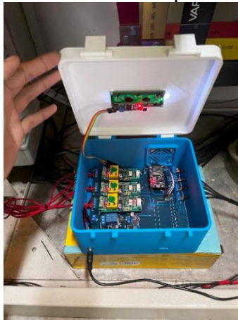
Gambar 8. Hasil alat monitoring mesin genset 300 kVA
