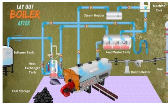
Gambar 6. Layout Boiler After
