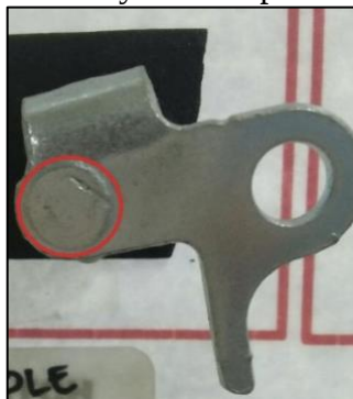
Gambar 3 Cacat No Hole
