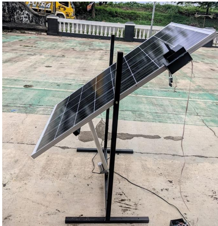
Gambar 1. Hasil Rancang Solar Panel Tracking
